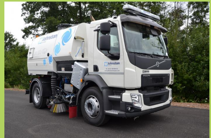
Street sweeper that meets the Euro 6 standard with effective PM collection equipment.
